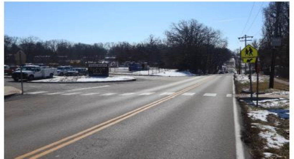
A Rectangular Rapid Flashing Beacon will be added at the mid-block crossing at Hanna Woods Elementary
